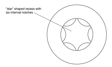
Figure 2.1 Torx Screw Identification
