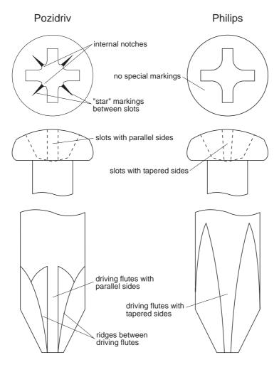
Figure 2.2 Pozidriv & Philips Screw & Screwdriver Identification
