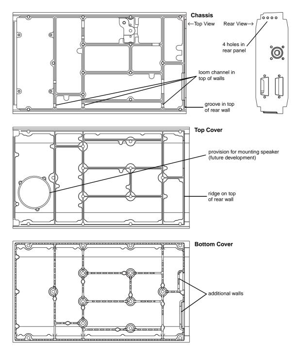
Figure 2.3 Identification Of New-Design Chassis & Covers
